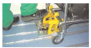
FIGURE 4. Releasing the trolley.
